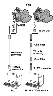
When connecting the camcorder to a PC using a DV cable, make sure to follow the procedure below. Connecting the cable incorrectly may cause malfunctions to the camcorder and/or the PC.
